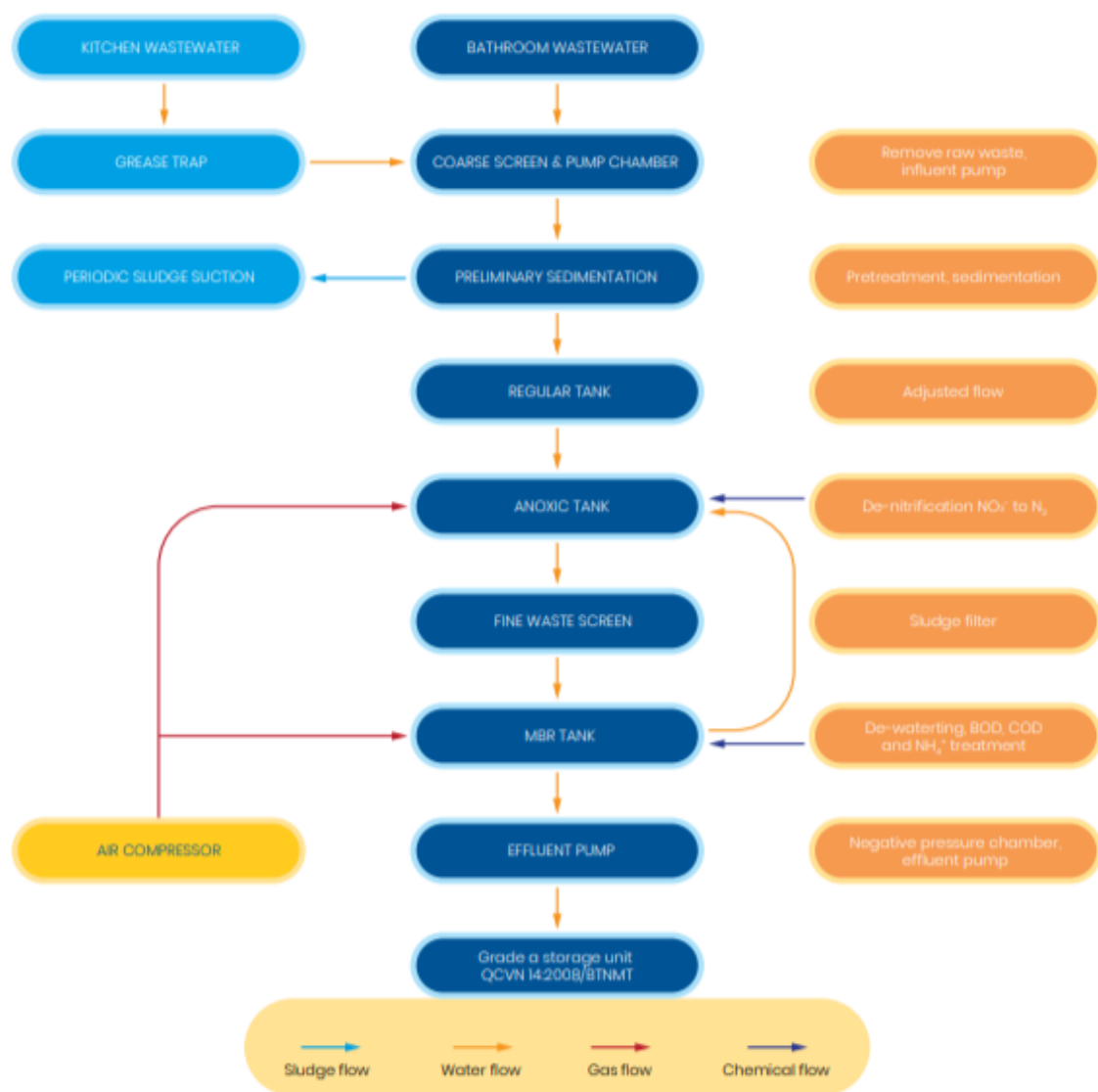
Diagram of the technology system for domestic wastewater treatment
